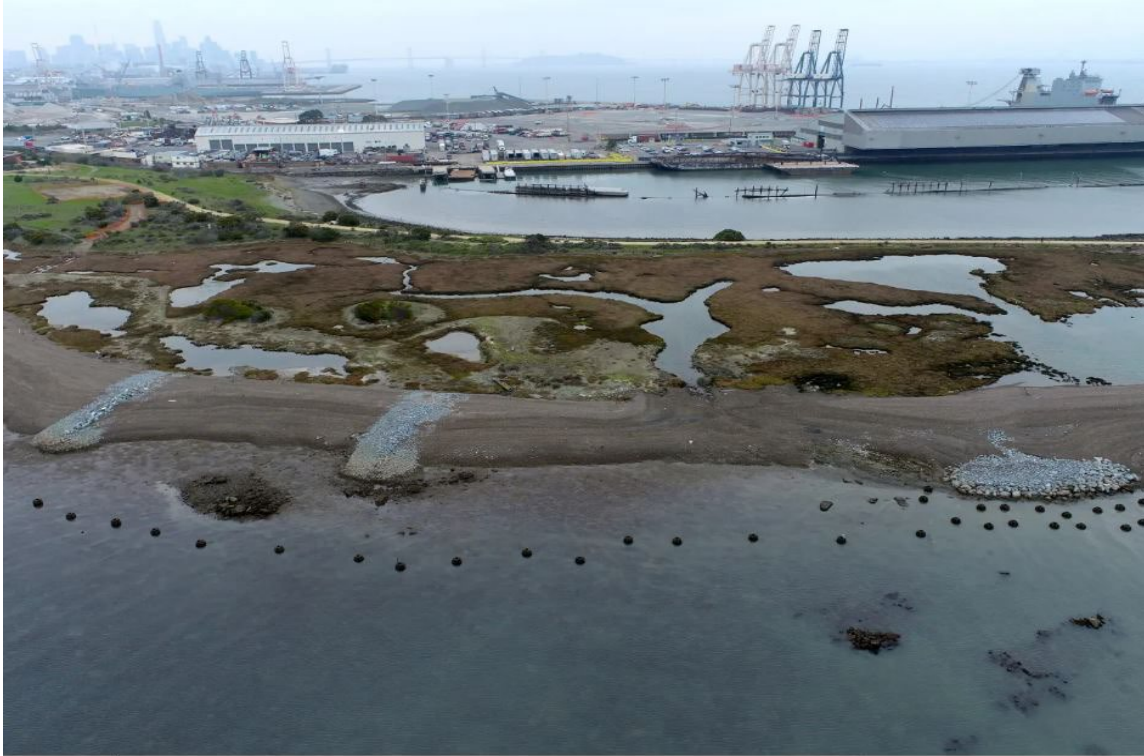
Figure I-10: Heron's Head Park, San Francisco highlighting wetland enhancement, and a coarse beach created to slow marsh edge erosion
